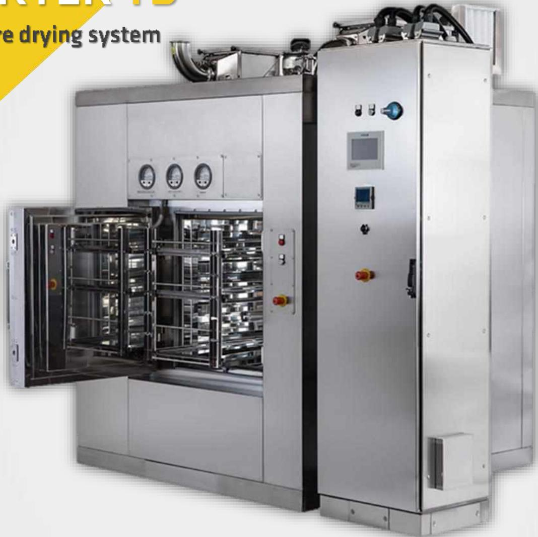
TD is designed for drying solid materials such as powders, fine granulates, machines parts, filters. The machine is provided with an integrated system of CIP or "isolated" filters equipped of "bag-in" and "bag-out" system. ATEX version also available.
